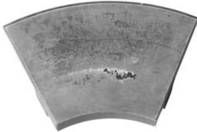
Figure 23 Thrust Shoe Cavitation Damage In Babbitt Face
