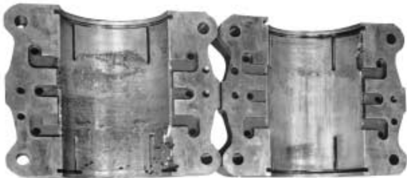
Figure 21 Edge Load Journal Shell with Babbitt Mechanical Fatigue
