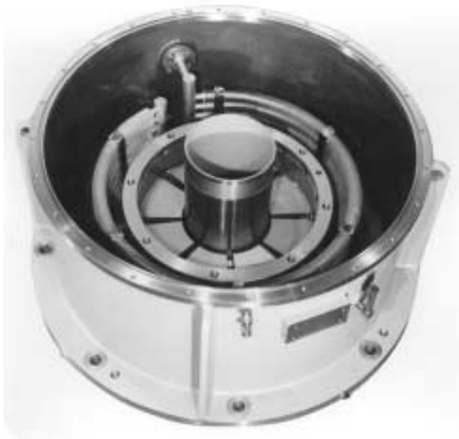
Figure 14 Vertical Thrust Bearing Oil Sump and Cooling Coils.
