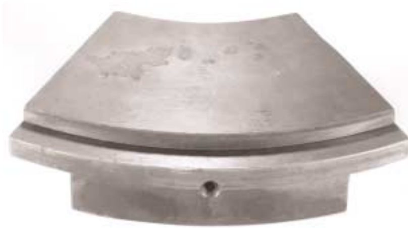
Figure 16 Tin Oxide Damage
