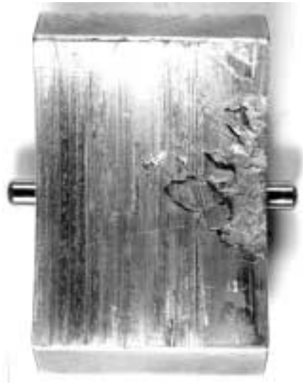
Figure 20 Edge Load Pivoted Shoe showing Babbitt Mechanical Fatigue
