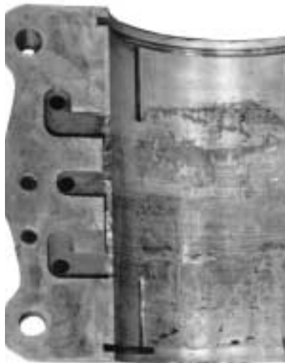
Figure 19 Stray Shaft Currents/ Electrical Pitting (Frosting).
