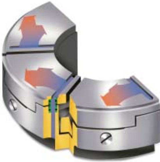
Figure 12 Leading Edge Groove Lubricant Flow Path.
