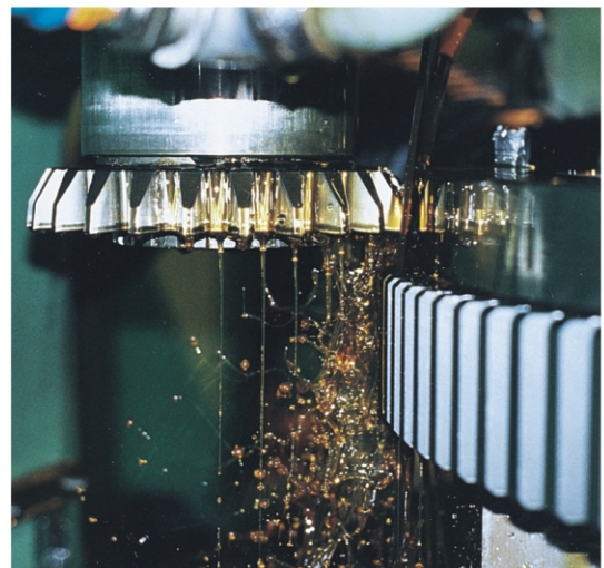
Internal and external gears can be cut to precision levels meeting AGMA Class 10.
