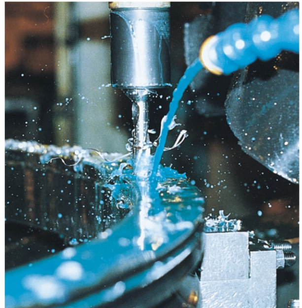
Special CNC machining centers drill bolt holes for mounting.
