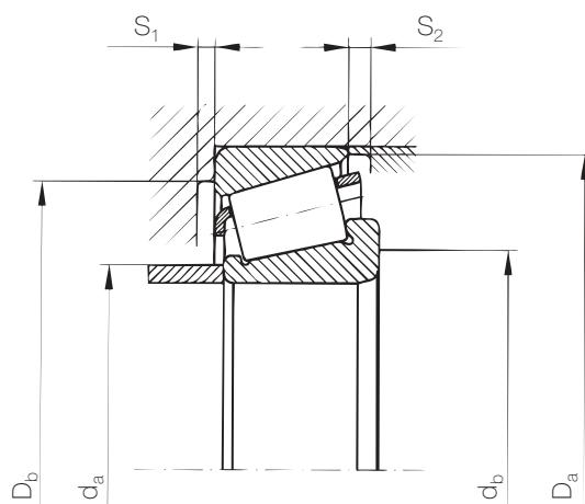
**NOTE:** For each bearing, Fersa has defined specific mounting dimensions which are provided when requested (db, da, Db, Da, S1, S2).
