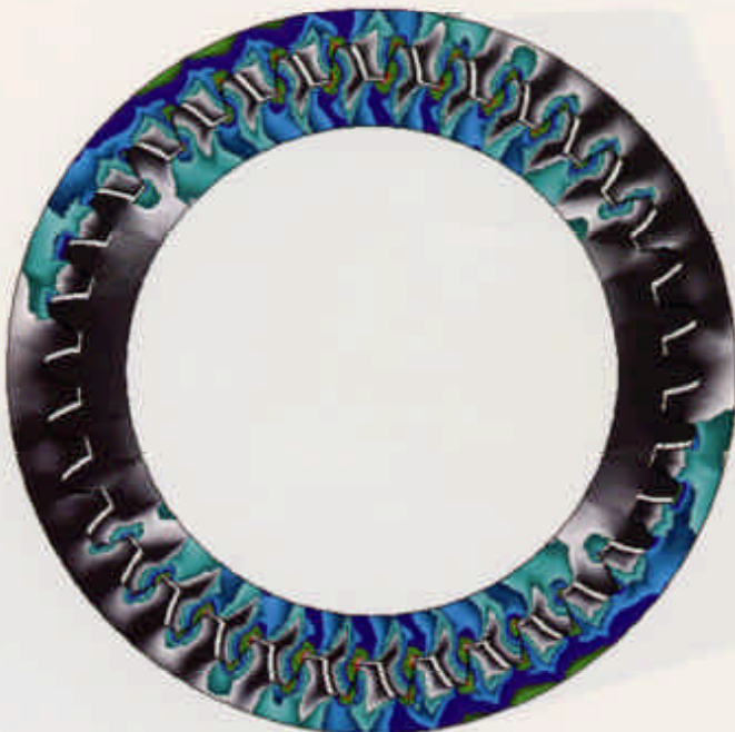
360° 2-D model at angle providing bending stress and percent of teeth in contact.
