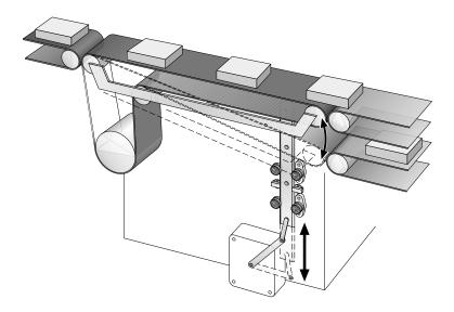
**SL2 System** is used as the vertical guidance in a food industry application to move a diverting conveyor between two further conveyors alternately. High speed and high duty operation driven by a crank arm.
