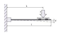
The deflection of a Slide beam acting as a cantilever and using a Long Flange Clamp (as shown opposite), will be a maximum at the free end when the load is at the outermost extremity of its stroke. This maximum deflection is given by the following equation:
