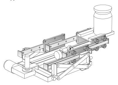
**SL2 System** is used for telescopic horizontal guidance in a Nuclear Industry drum handling application. Vertical movement is provided by a scissor lift.
