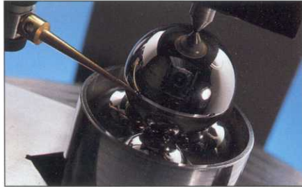
Control of ball geometry helps reduce bearing vibration levels.
