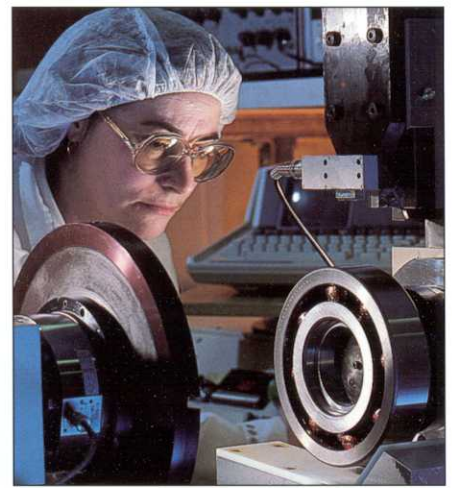
The unique, Barden-designed "Quiet Bearing Analyzer" allows functional testing of bearings at thrust loads rated well beyond those of commercially available bearing testers.
