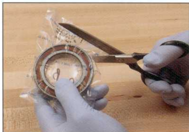
Open package with scissors. Handle only with clean, dry hands or gloves.
