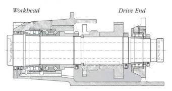
Heavy-duty lathe spindle showing a double direction angular contact thrust ball bearing used with a double row cylindrical roller bearing in the workbead. Drive end of the spindle features one double row cylindrical bearing. This combination allows spindle to operate with high rigidity, while accommodating both axial and radial loads.
