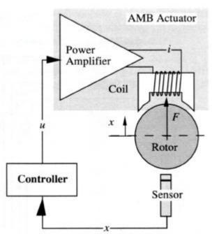
The main components required for a full five axis system (i.e. A system that controls five degrees of freedom) are shown below.
