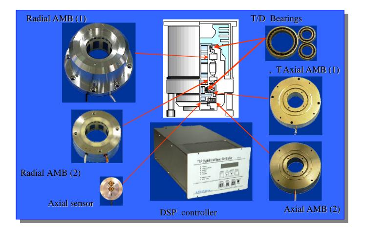
By using two radial bearings and two axial bearings it is possible to control exactly the spindle position at all times. The emergency touchdown bearings will support the shaft in case of complete power failure and allow the shaft to coast to a stop in a controlled manner.
