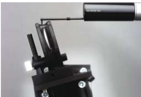
Curvature inspection of an inner raceway.
