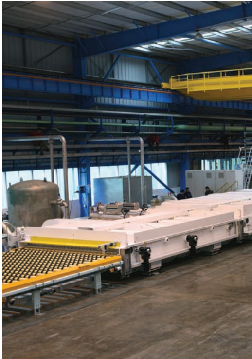
Glass coating unit for coating of glass with LowE- and Solar-Control-Coating
