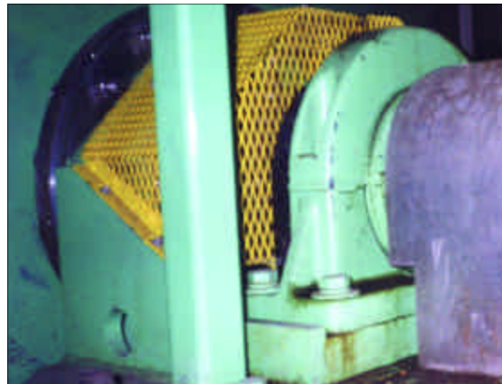
Take Up Tension Type 1 3/16" / 30mm to 6" / 155mm Available in cast iron Also offered as push type
