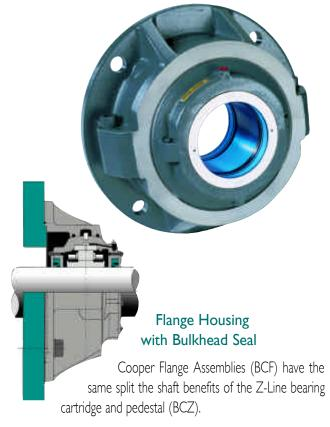
Bulkhead sealing is achieved by an 'O' ring in the rear face of the flange housing. This sealing is proven effective where bulkheads are not loadbearing and Cooper flange assemblies have been specified as bulkhead seals.
