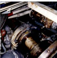
The Cooper bearing is easy to fit into confined spaces on board vessels of all sizes with easy access for propulsion shafting maintenance and inspection, gives more uptime and lower maintenance, inspection and replacement costs.
