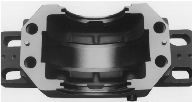
Large capacity oil sump lowers operating temperatures. Undercut bearing seat allows full lateral travel of expansion bearing. Prevents stabilizer ring from binding, makes installation easy.
