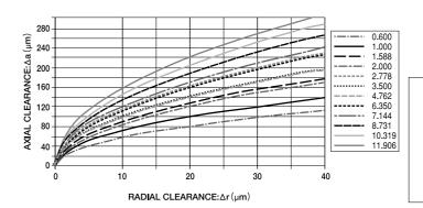
$\Delta a = 2\sqrt{\Delta r(r_0 + r_1 - Da)}$  (mm)
