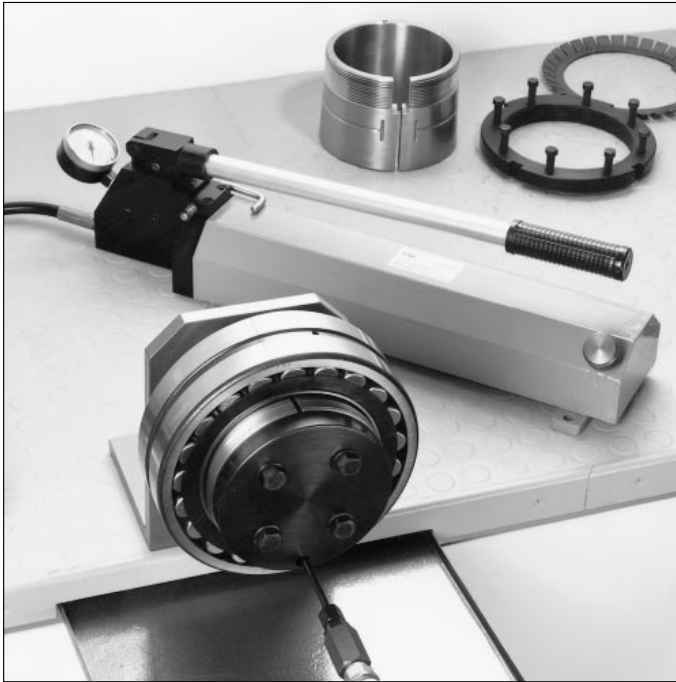
56: Mounting of a tapered bore spherical roller bearing by the hydraulic method
