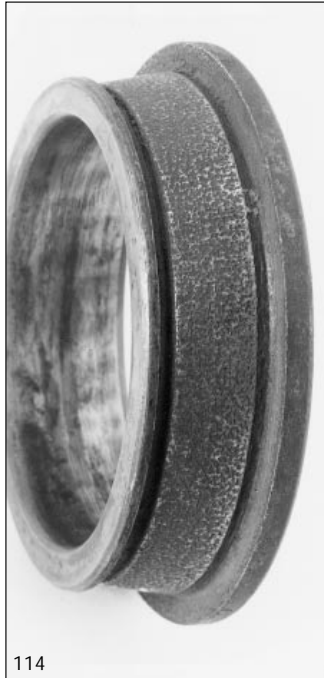
115: Corrosion marks in the raceway of a self-aligning ball bearing outer ring
