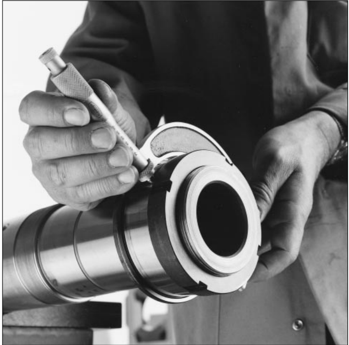
29: Measuring the expansion of a cylindrical roller bearing inner ring with an external micrometer
