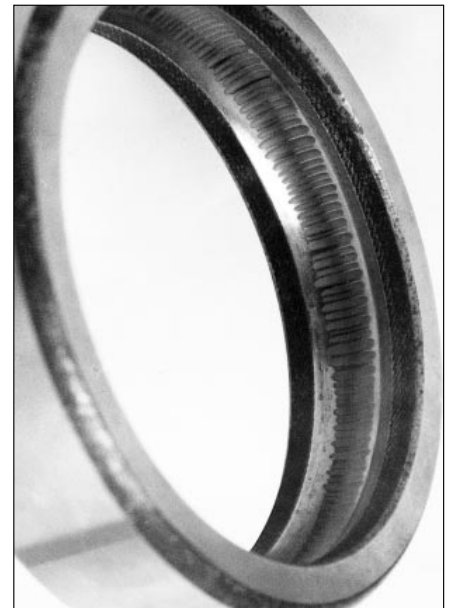
60: Fluting in the outer ring raceway of a deep groove ball bearing was caused by the constant passage of current.
