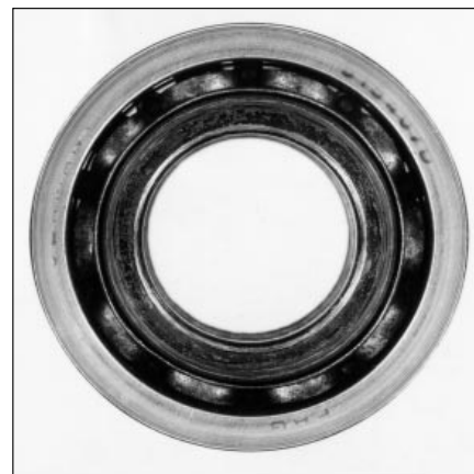
17: Circumferential scoring and cold welding at the inner ring faces as a result of inner ring creeping on the shaft
