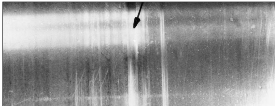
70: Deep scratches on rollers as a result of foreign particles in the cage
