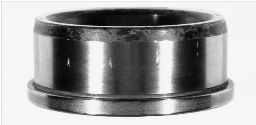
76: Score marks in the raceway of a cylindrical roller bearing inner ring caused by out-of-square insertion into the rolling element set
