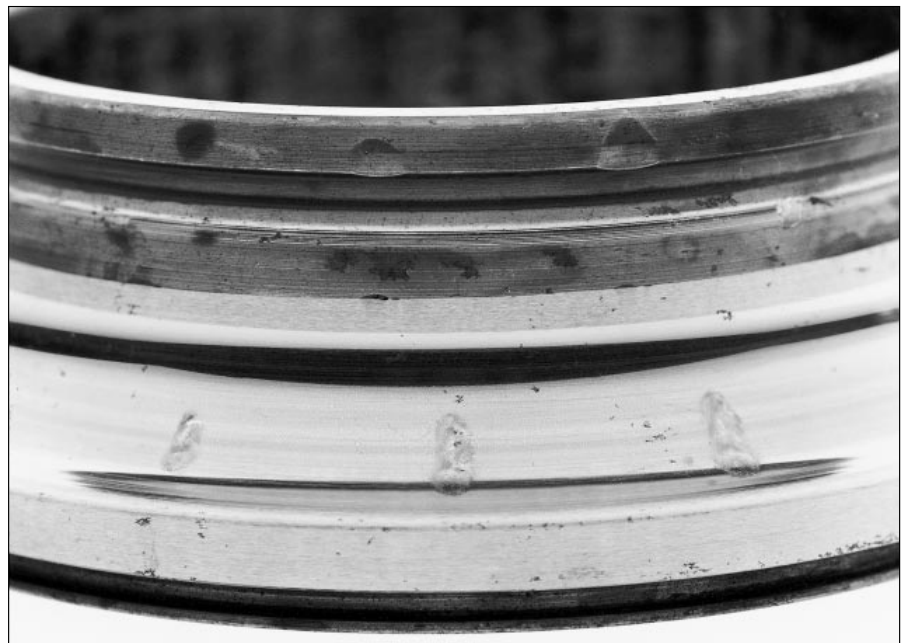
57: False brinelling on the ball bearing
