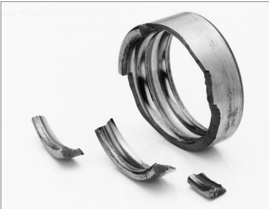
65: Crack in outer ring in circumferential direction
