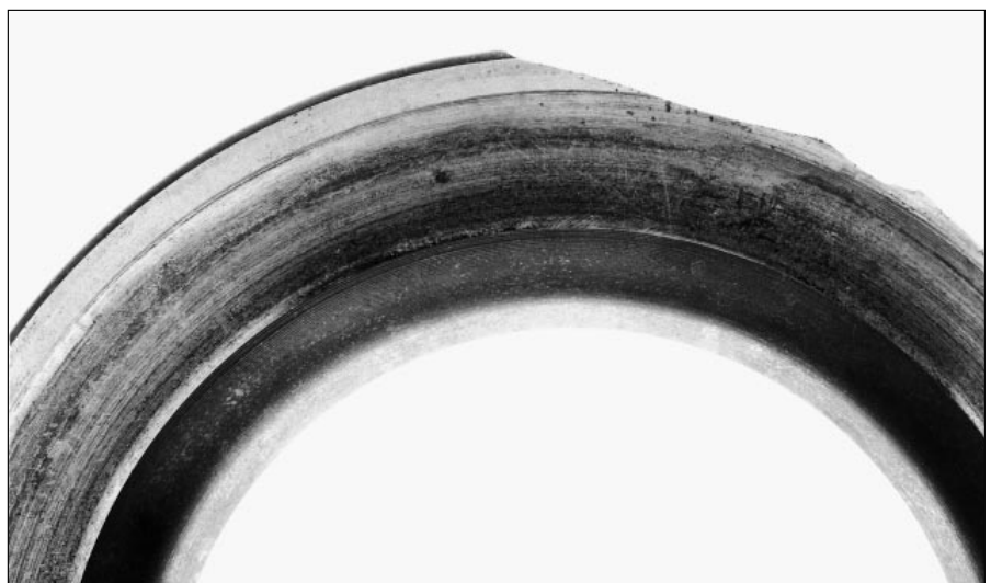
20: Lip fracture of a tapered roller bearing cone due to insufficient axial support of face
