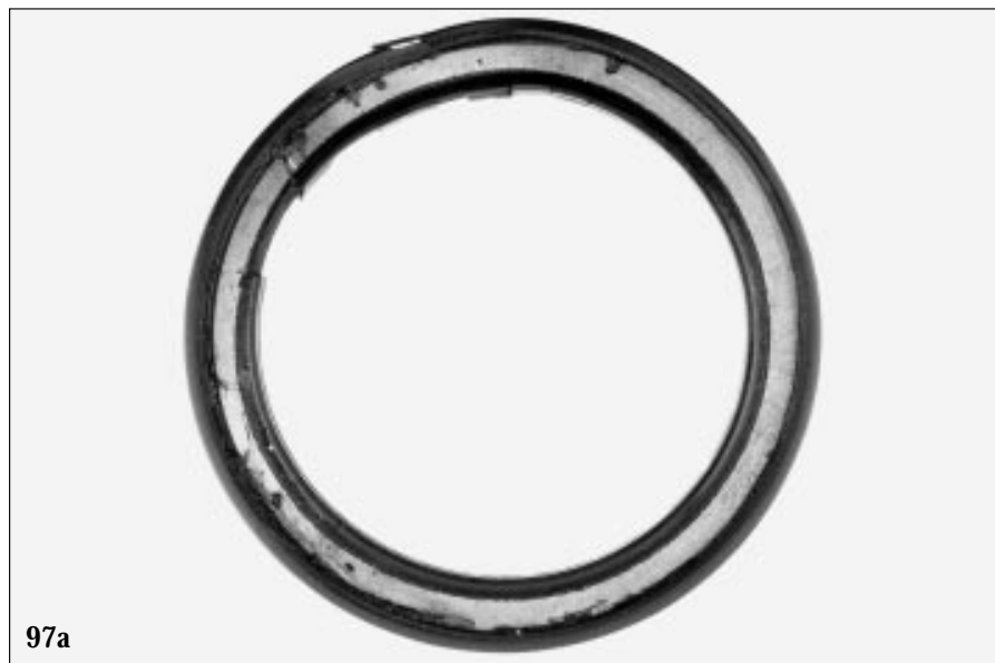
97: a: Hardened sealing with wear and fractures
