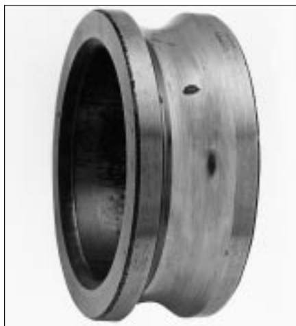
41: Classical fatigue can be recognized by pitting in the raceway of a deep groove ball bearing inner ring. Material flakes off the entire raceway when damage advances.
