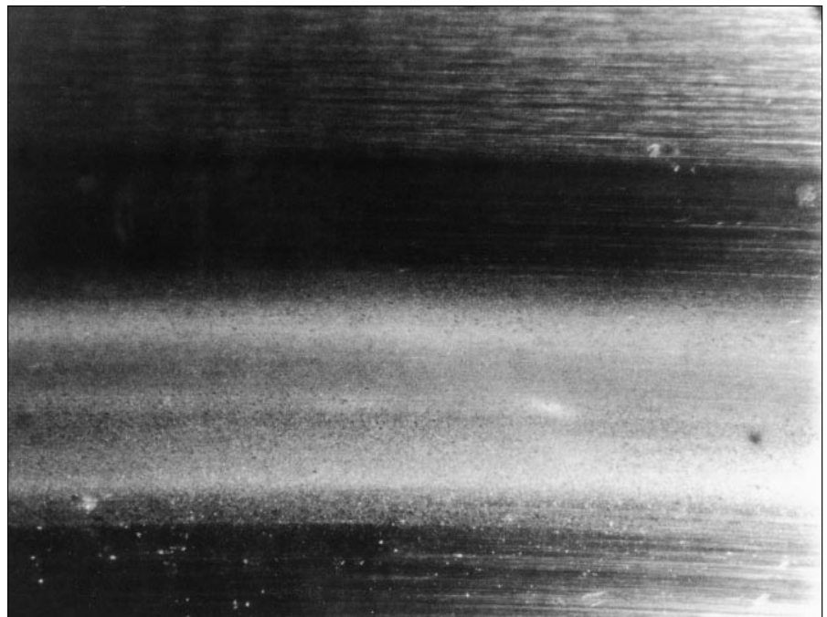
66: Worn, roughened raceway
