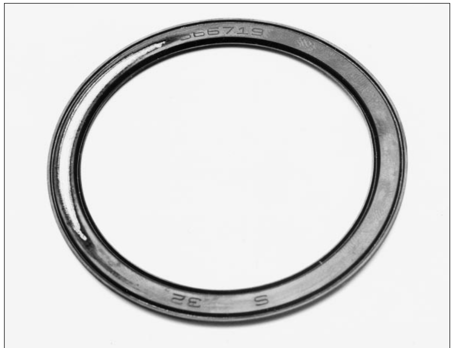
22: Seal damage due to lateral grazing
