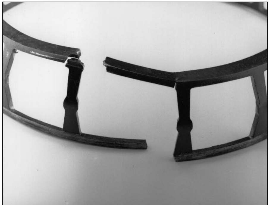
93: Disruptive fracture at the side edge of a spherical roller bearing cage
