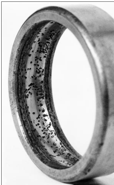
53: Corrosion of the outer ring of a deep groove ball bearing, the corrosion protection of which was destroyed by humidity
