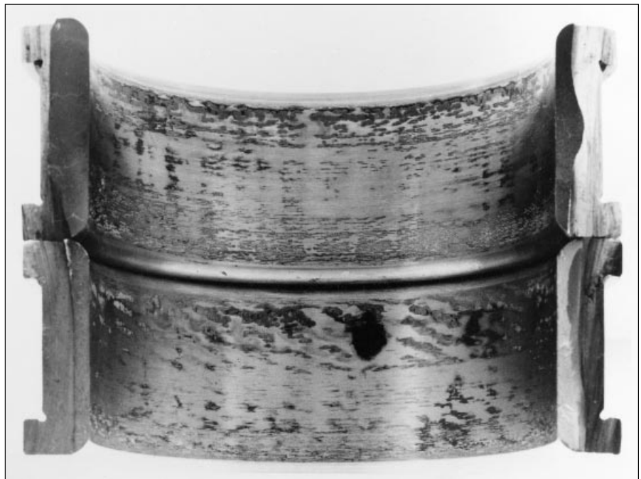
13: Fretting corrosion in bore of a cylindrical roller bearing inner ring with seat too loose
