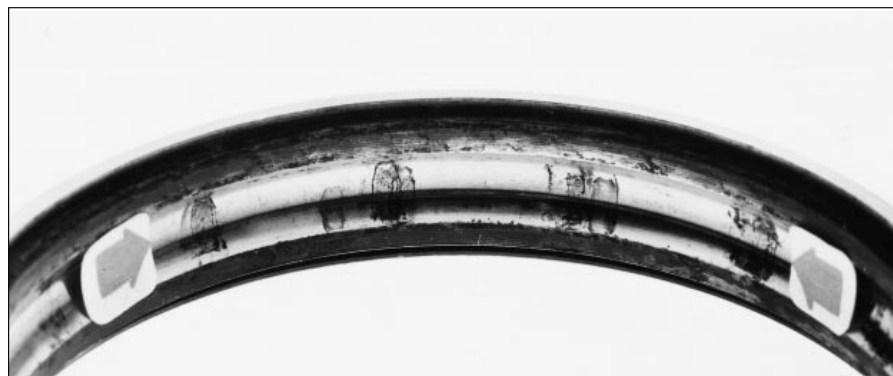
54: Corrosion pits in the raceway at rolling element pitch
