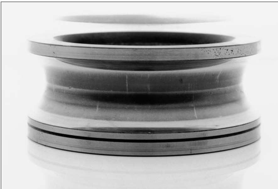
28: Track with surface wear
