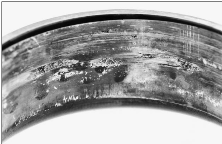
16: Seizing marks in the inner ring bore as a result of inner ring creeping on the shaft
