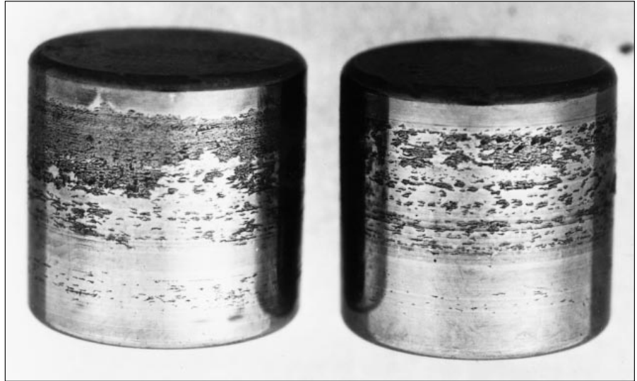
74: Slippage tracks on cylindrical rollers
