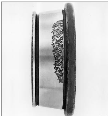
40: Tilted track on a tapered roller bearing
