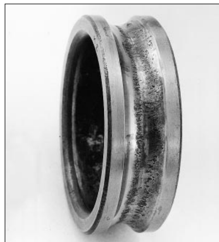
42: Advanced fatigue damage on deep groove ball bearing
