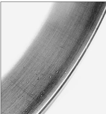
23: Normal track, surface structure still visible, just small indentations by foreign particles
