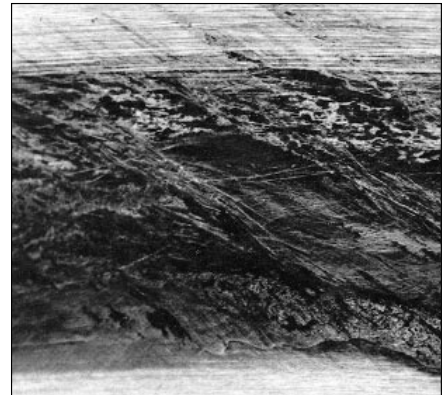
82: Seizure can arise at the roller face and lip when the lubricant supply is inadequate and loads are high.
