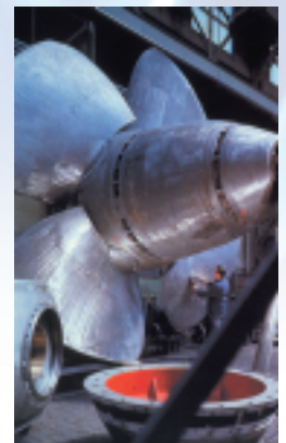
deva.bm®, deva.bm®/9P in turbine construction: Kaplan turbine: rotor blade adjustment
