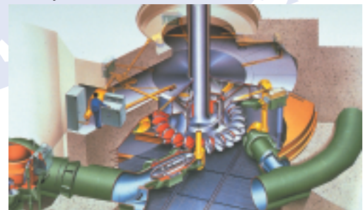
deva.bm®, deva.bm®/9P in water turbine construction: Pelton turbine: nozzle valve, jet deflector
