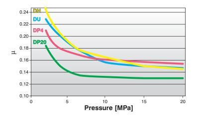
Dry friction under low speed conditions: Speed: 0.04 m/s
