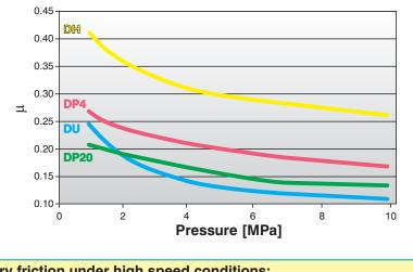
Dry friction under high speed conditions: Speed: 0.7 m/s
