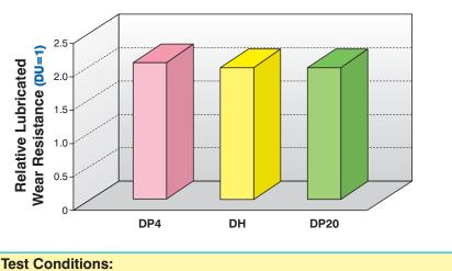
Speed: 0.11 m/s Load: 12 - 40 MPa Lubricant: BP Bartran HV
