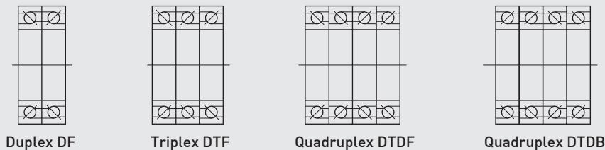
Fig 4.4 Different arrangement of ballscrew support bearings
