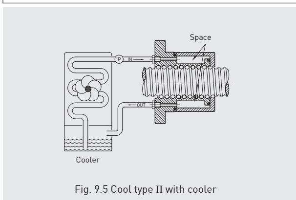
Fig. 9.5 Cool type II with cooler
