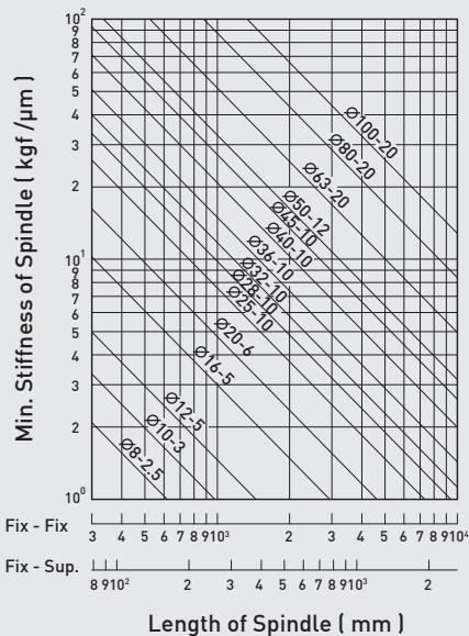
Fig 4.28 Stiffness chart for ballscrew spindle
