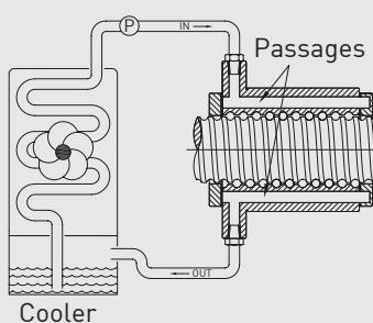
Fig. 9.2 Cool type I with cooler
