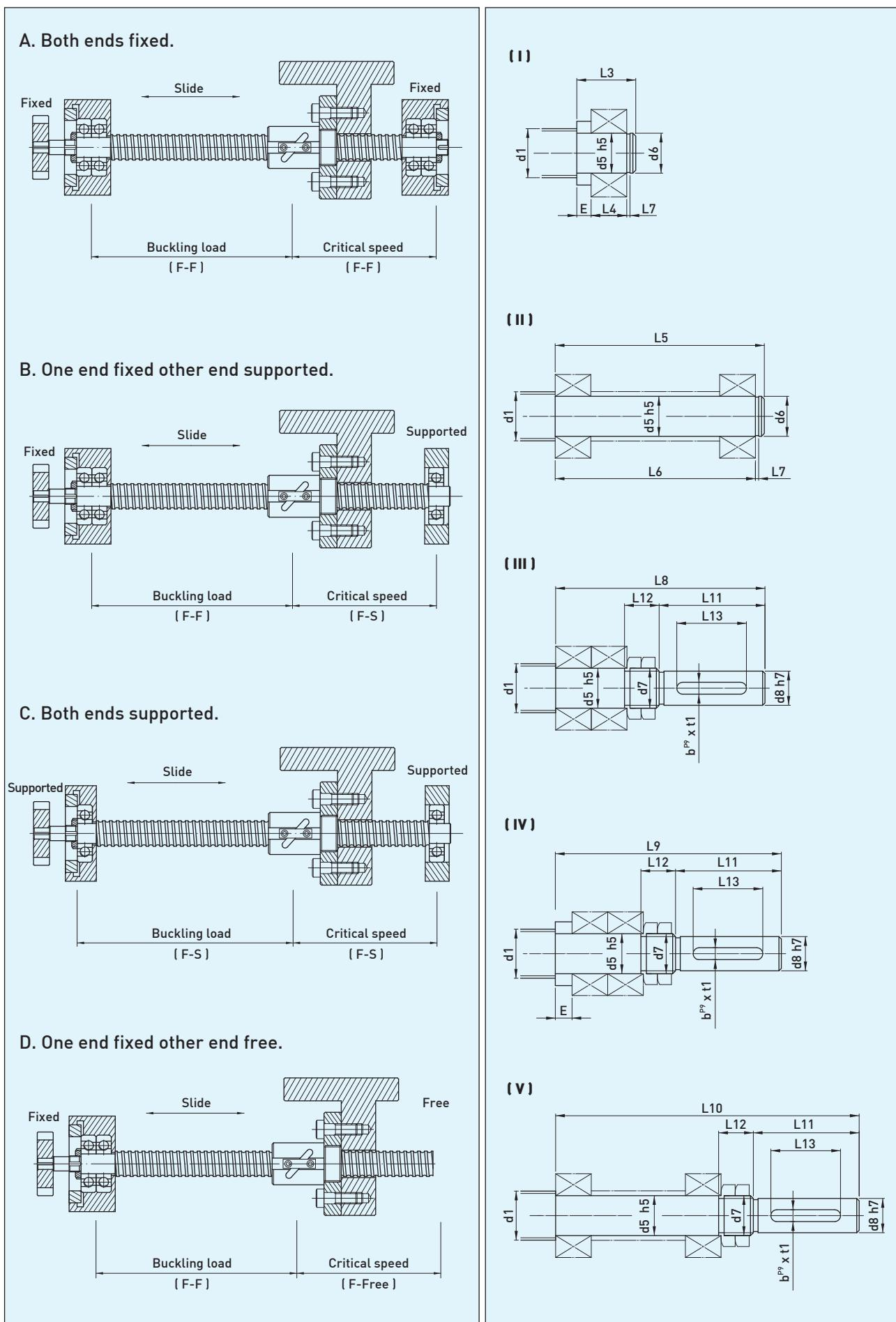
Fig 3.6 Recommended mounting methods for the ballscrew end journals
