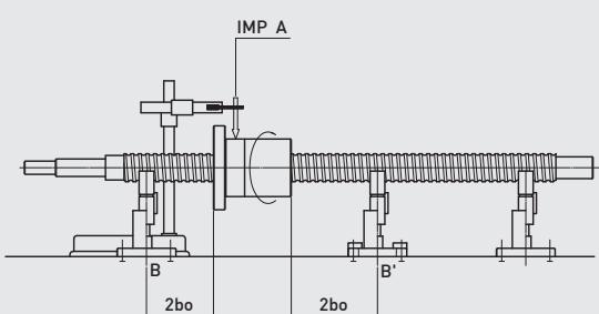
T6 : Run-out deviation of external diameter (only for nut) relative to BB' (This measurement is made according to DIN 69051 and JIS B1192)
