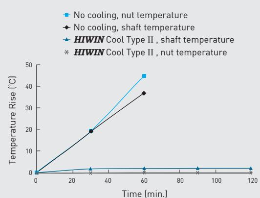
Fig. 9.6 Cool type II : Temperature rise of ballscrew
