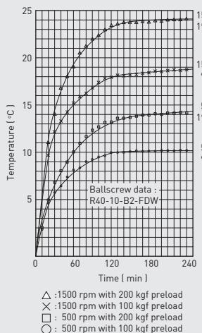
Fig 4.29 The relation of working speed, preload and temperature rise
