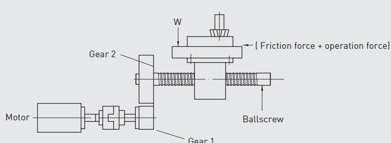
Fig 4.23 Load operation by ballscrew
