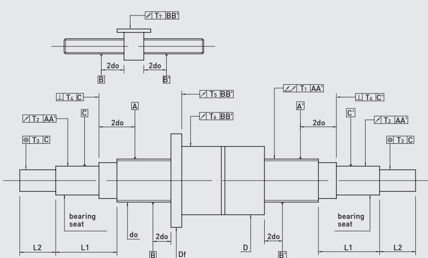
Fig 4.15 Geometrical tolerance of HIWIN precision ground ballscrew
