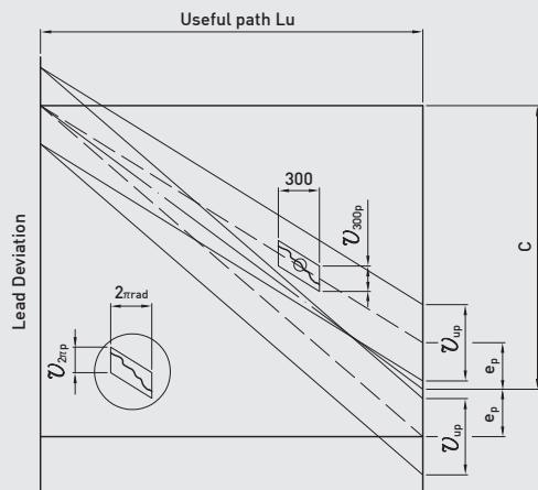
Fig 4.13 DIN lead measuring curve of precision ballscrew
