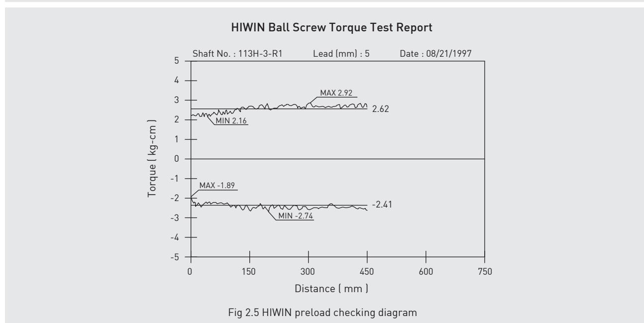
Fig 2.5 HIWIN preload checking diagram
