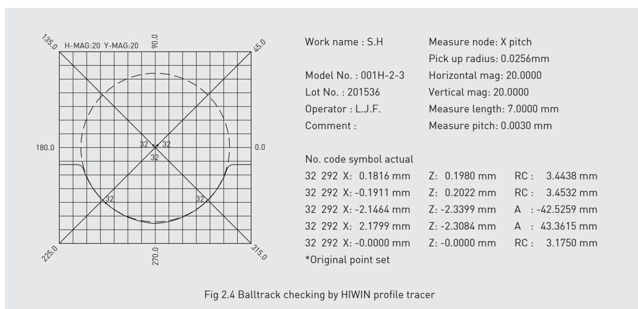
Fig 2.4 Balltrack checking by HIWIN profile tracer
