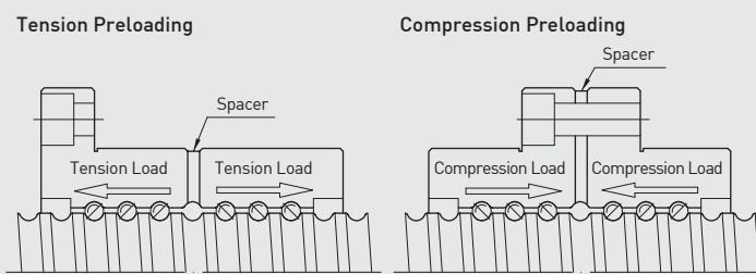
Fig 4.17 Preload by spacer
