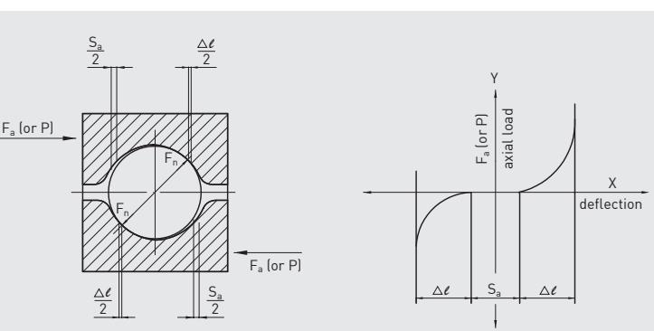
Fig 4.16 Gothic form profile and preloading relation
