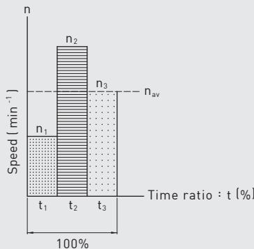
Fig 4.22 Equivalent speed
