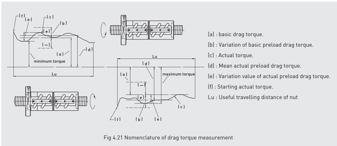
Fig 4.21 Nomenclature of drag torque measurement
