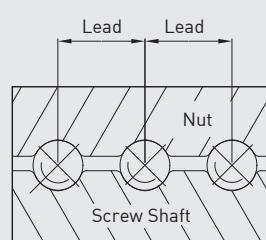
Fig 4.18 Preload by ball size
