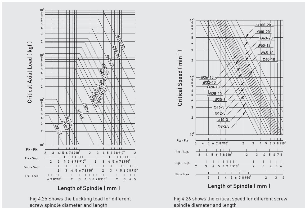
Fig 4.25 Shows the buckling load for different screw spindle diameter and length
