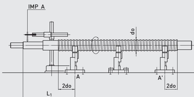
T2: Run out deviation of bearing relative to AA' (This measurement is made according to DIN 69051 and JIS B1192)
