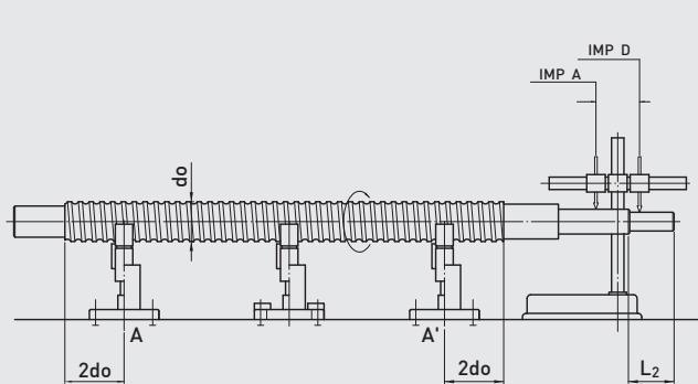
T3: Coaxial deviation relative to AA' (This measurement is made according to DIN 69051 and JIS B1192)
