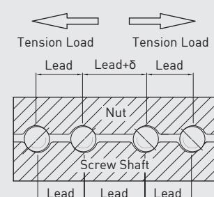
Fig 4.19 Offset type preloading
