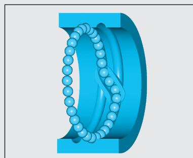
Fig 3.5 Circuit for internal return cap
