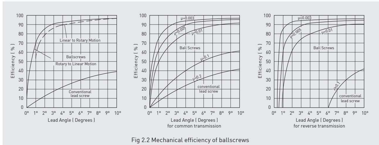
Fig 2.2 Mechanical efficiency of ballscrews
