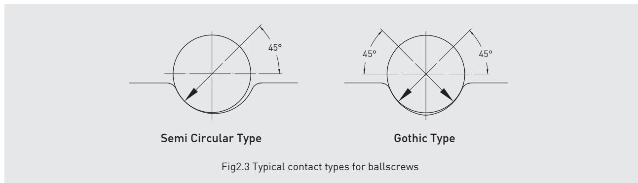
Fig2.3 Typical contact types for ballscrews
