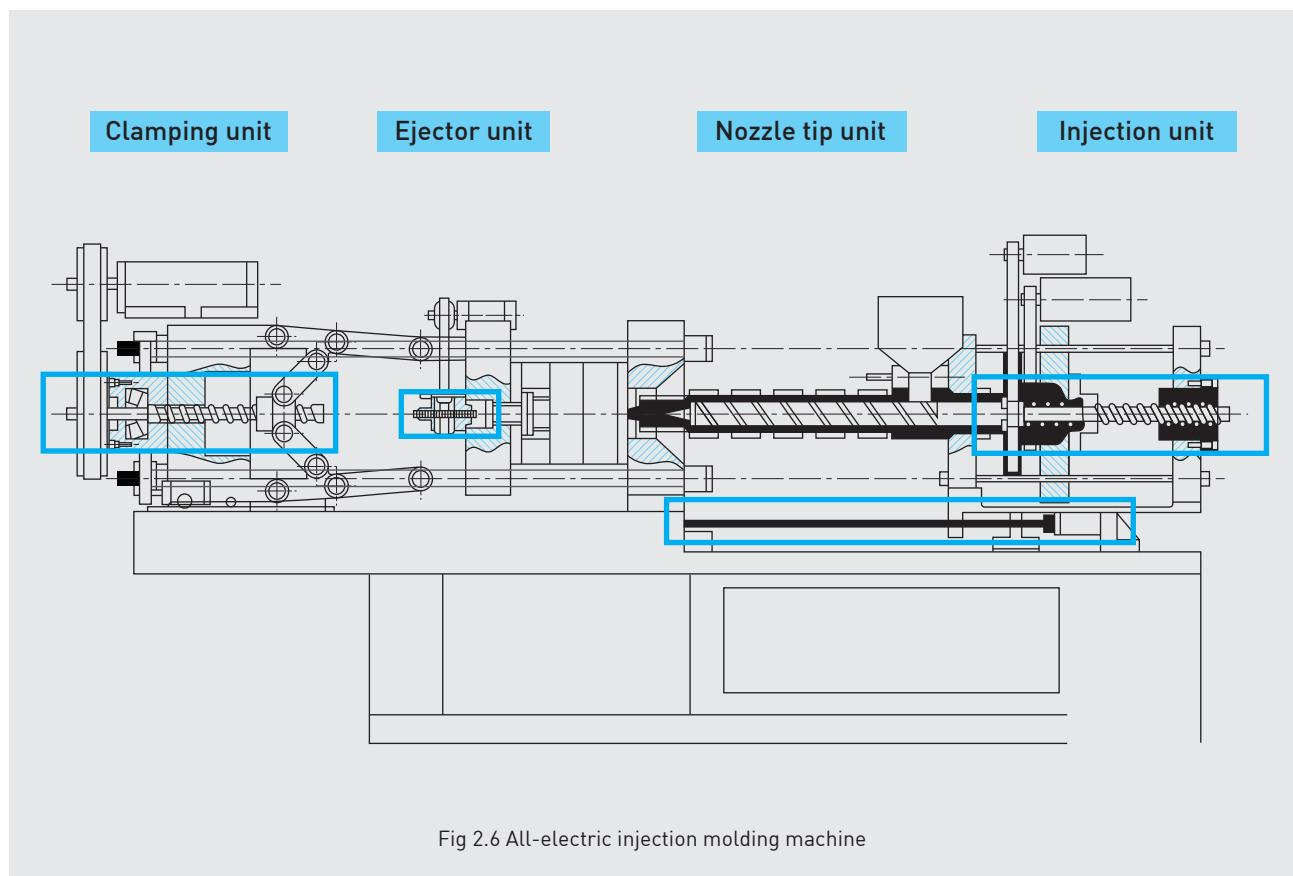
Fig 2.6 All-electric injection molding machine
