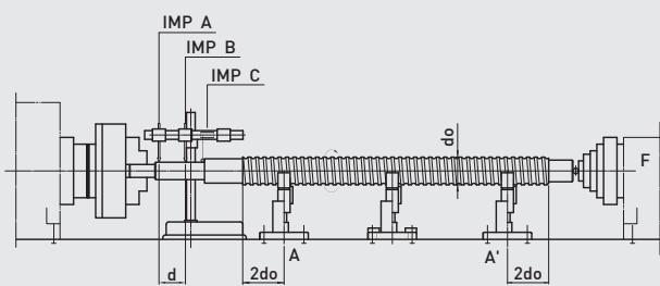
T4 : Run-out deviation of bearing end shoulder relative to AA' (This measurement is made according to DIN 69051 and JIS B1192)
