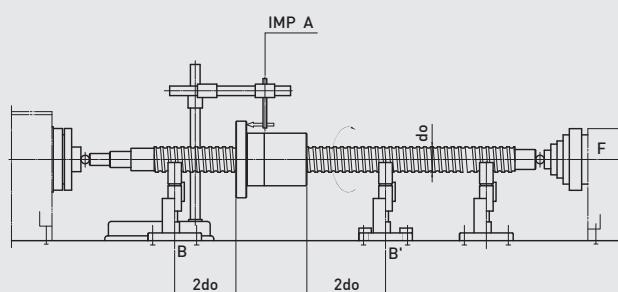
T5 : Face running deviation of locating face (only for nut) relative to BB' (This measurement is made according to DIN 69051 and JIS B1192)
