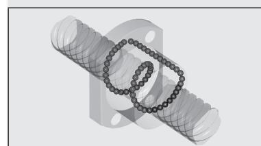
Fig.3.3 Endcap recirculation type nut with return system
