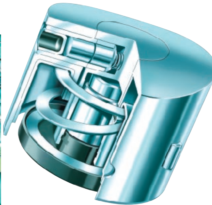
Hydraulic camshaft phaser with timing chain sprocket. Its job: to ensure precise and continual adjustment for valve timing with a large torsional angle
