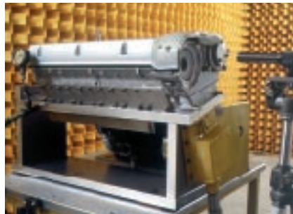
Acoustic analysis of an engine in an anechoic chamber. INA testing facilities are equipped with state-of-the-art technology
