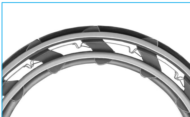
Fig. 6.2 One-way Clutch in Pop-out State
