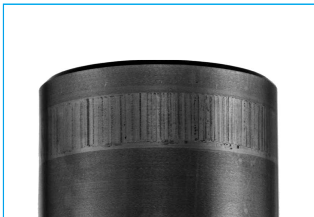
Fig. 6.3 Sliding Nicks on the Inner Ring Raceway Caused by Popping
