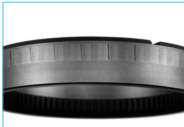
Fig. 6.5 Brinelling on the Inner Ring Raceway Surface Caused by Roll-over
