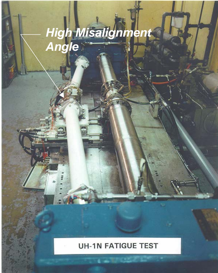
Kamatics KAflex endurance test rig showing the high misalignment capability of the KAflex design.
