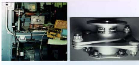
Reversing torque Test and the Tested Coupling
