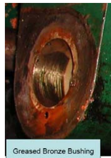
Greased Bronze Bushing After 10 years of Service
