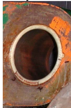
KARon Linkage Bushing After 10 years of Service
