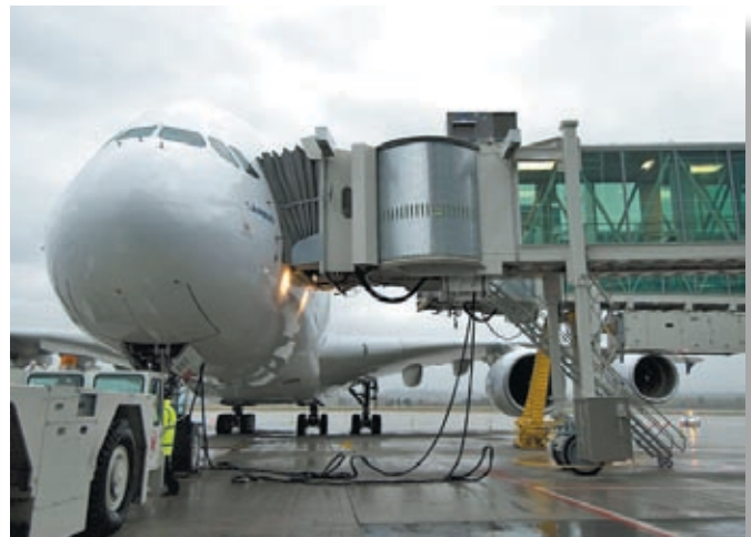
FMC Jetway Apron Drive Passenger Boarding Bridge. © 2007 Photo by P.Michaud. Courtesy of FMC Technologies, Jetway.
