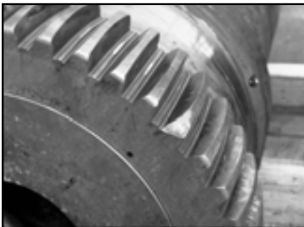
Tooth End Breakage due to over-misalignment
