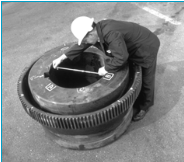
KOP-FLEX service technician inspecting gear coupling
