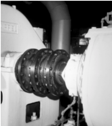
FAST'S® Gear Coupling Size 8-30
