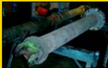
A universal joint, as received from a customer, at our service center for inspection and rebuilding
