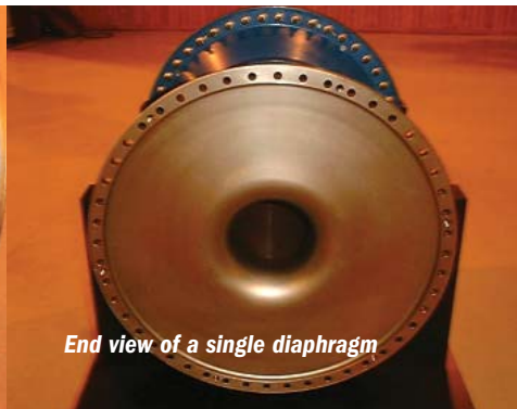
Figures 4, 5, 6: Diaphragm couplings accommodate flexure from the metal between its outside and inner diameter
