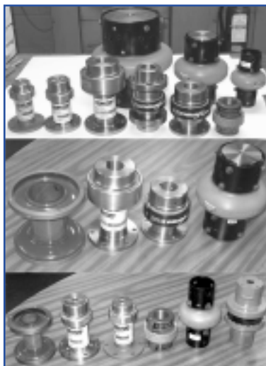
Figure 5. Miscellaneous types and sizes of couplings tested, including dual-flex elastomeric diaphragm, urethane tyre, unclamped donut, jaw in shear and wrap-jaw.
