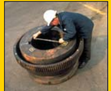
KOP-FLEX service technician inspecting gear coupling
