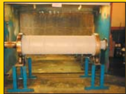
LM 2500 gas turbine coupling after complete refurbishment
