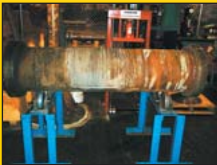
LM 2500 gas turbine coupling before being refurbished
