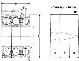
The PumPac 8000-AAB series consists of two 40  $^{\circ}$  (A) and one 15  $^{\circ}$  (B) bearing.
