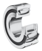
LAMBDA<sup>®</sup> sealed SPHERE-ROL<sup>®</sup> bearings should not be operated at misalignment angles in excess of  $\pm 1^{\circ}$  and for best seal efficiency, operating misalignment angles should not exceed  $\pm 1/2^{\circ}$ . The LAMBDA<sup>®</sup> seal should not be operated at temperatures exceeding 300°F. Please consult the McGill Engineering Department when higher temperatures must be considered.
