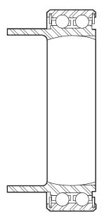
Double Row Ball Bearing Helicopter Main Rotor Swashplate
