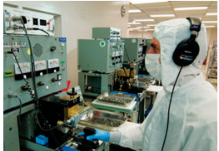
Anderometer, Dynamic Noise and Vibration Tester
