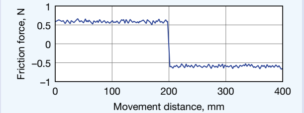
Fig. 2-1 Fluctuations in dynamic friction
