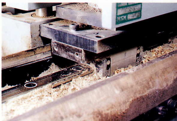
Fig. 60 Durability test of linear guide exposed to wood chips
