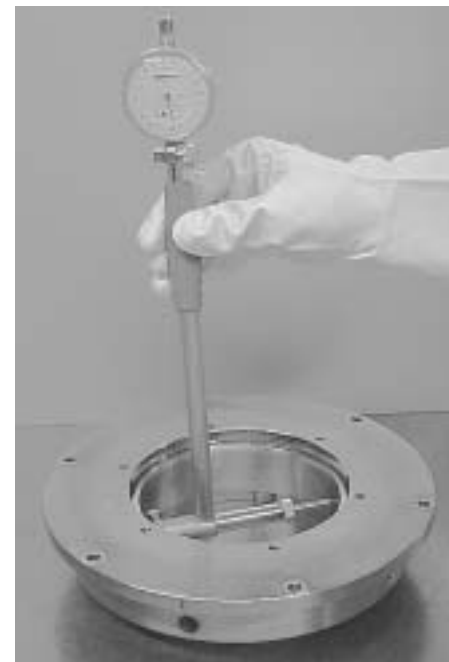
Fig. 1.10 Zero Setting of Cylinder Gauge
