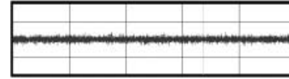
Sound waveform of a normal bearing
