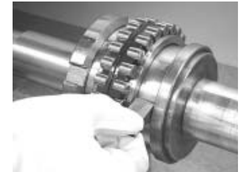
Fig. 1.15 Measurement of Spacer Width
