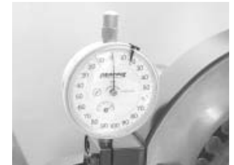
Fig. 1.15 Measurement of Spacer Width
