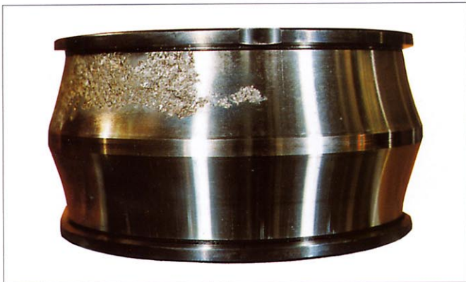
Photo 7-1-9 Part: Inner ring of a spherical roller bearing Symptom: Flaking of only one row of raceway Cause: Poor lubrication
