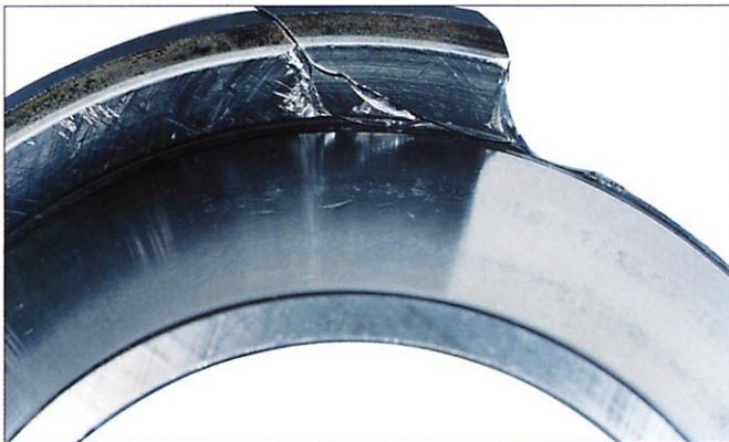
Photo 7-5-3 Part: Inner ring of a spherical thrust roller bearing Symptom: Fracture occurs at the large rib Cause: Repeated load
