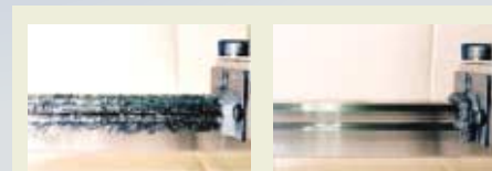
Before passage of ball slide (Significant foreign matter remains after passage of the slider) After passage of ball slide (All foreign matter is swept away)
