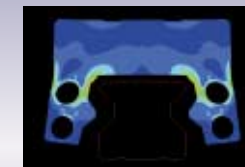
Example of roller slide deformation analysis
