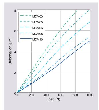
Figure 4 Monocarrier's rigidity in radial direction
