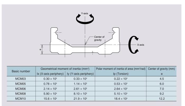
Figure 5 Rail moment of inertia
