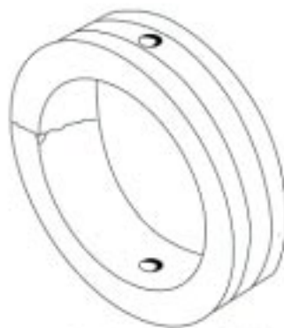
Figure 3: Single Fractured Outer Ring
