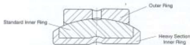
Figure 5: Standard vs. Heavy Section Inner Ring
