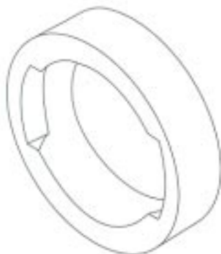
Figure 1: Outer Ring with Loading Slots
