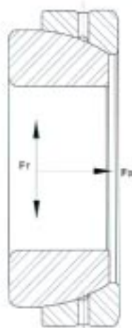
Figure 9: Angular Contact Bearing. Single Acting. Permissible Load Directions
