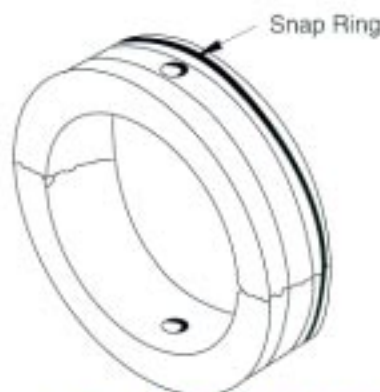
Figure 2: Double Fractured Outer Ring
