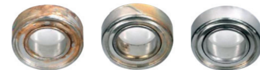
Regular steel after standard ISO test
