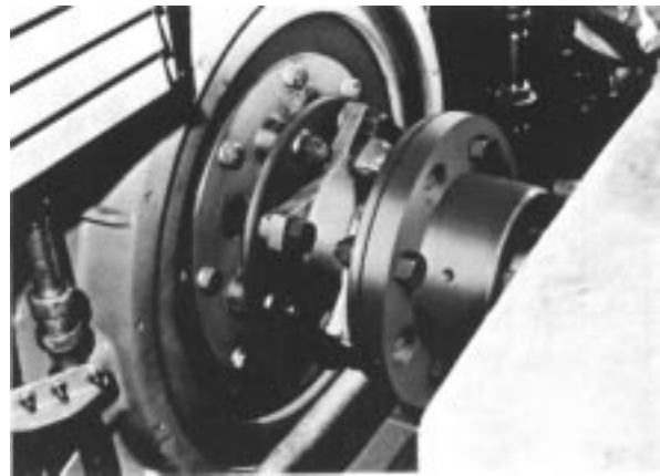
CMR coupling between engine and reciprocating compressor.
