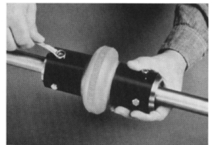
Mount other half of the Omega element. Tighten all capscrews to recommended torques below and you're done! Refer to the installation instructions for further details.
