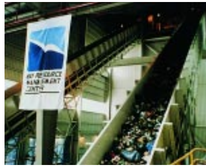
Rex Style A pan conveyor handling municipal solid waste.
