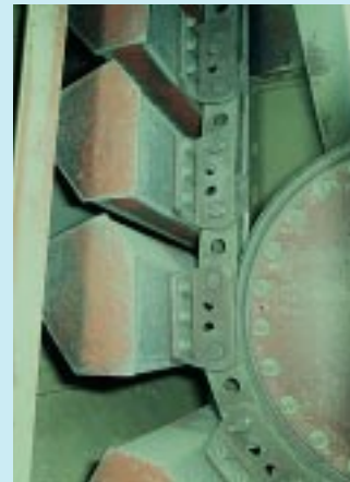
Rex single strand, high quality fabricated steel bushed chain.
