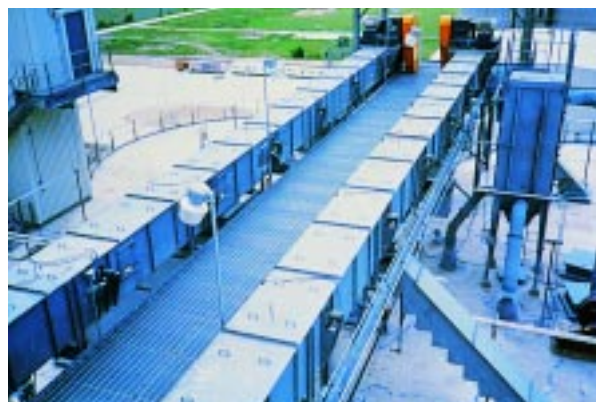
Drag conveyors used for feeding multiple discharge points.
