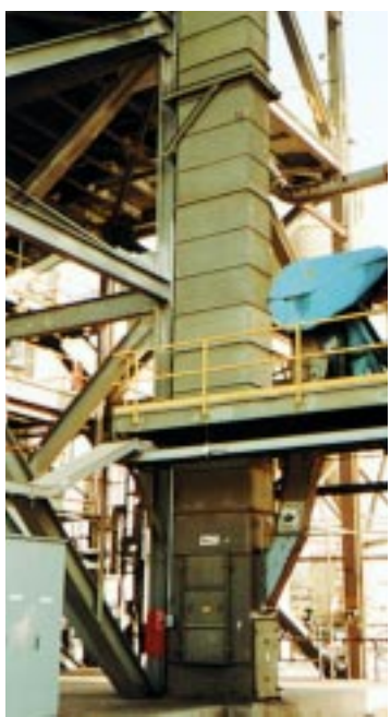
Rex chain bucket elevator for handling coal.
