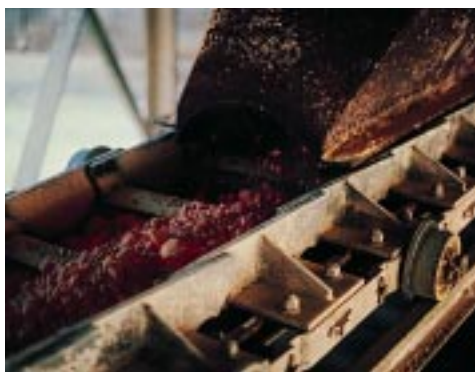
Rex pan conveyor for hot lime handling.
