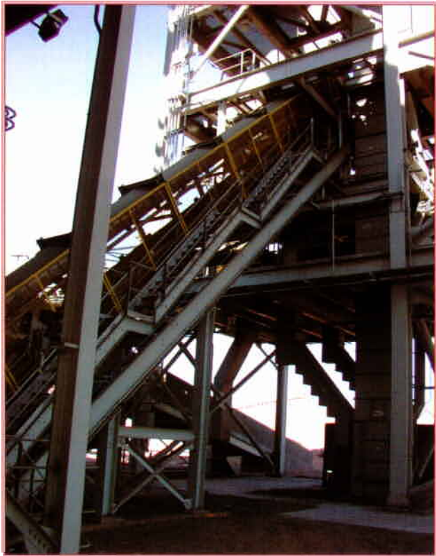
RexAFT pan conveyor and bucket elevator which handles clinker from the clinker cooler.
