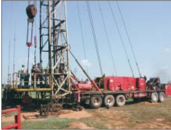
Pool Well Services' workover rig is experiencing longer life on roller chain used to drive the drums and other functions. Here, the 500 HP rig pulls tubing from an oil well near Oklahoma City.
