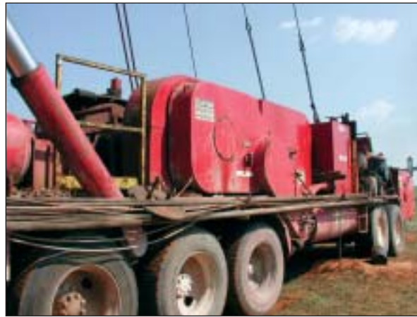
Closeup shows drum drive. Multiple-strand chains are inside guards.
