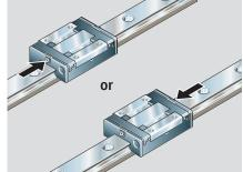
For **short stroke** applications, apply either the total amount as per table to each end-face lube nipple, or the partial amount per side as given in the table to each side lube port.
