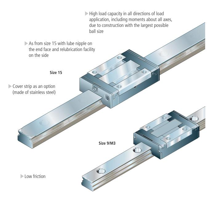
All steel parts of the runner block and the guide rail are made of rust and acid resistant material similar to ISO 683-17 / EN 10088
