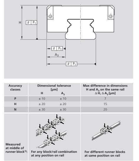
1) In dimensions H and  $\Delta$ H, the middle of the runner block is calculated from the mean of the two measuring points shown.
