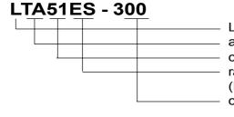
LIGHT RAIL Series aluminum telescopic rails characteristics external size rail locked when fully extended (ES for left rail or ED for right rail) closed length
