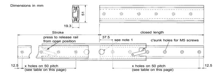
note 1: Ø15 mm holes in center beam allow easy access to fixing holes.
