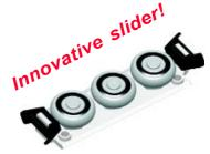
The contoured rail comes in lengths up to 3 meters (9'10"). The raceways are internal for better protection and compactness. The rails come with standard mounting holes with a hole pitch of 80mm (3.15"). The steel rollers have 2Z sealing and are lubricated for life. These rollers have eccentric pivots that allow adjusting the preload when mounted inside the rail.
